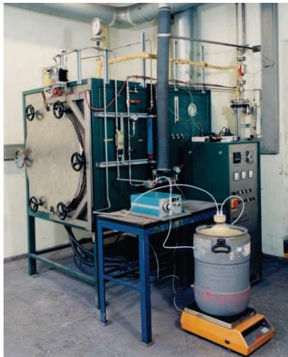
*Special furnace for catalytic debinding
