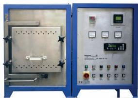
*HT-1600-G-Graphite (Tmax 1600 °C, optional up to 2200°C). Protective gas and vacuum tight, different sizes*
